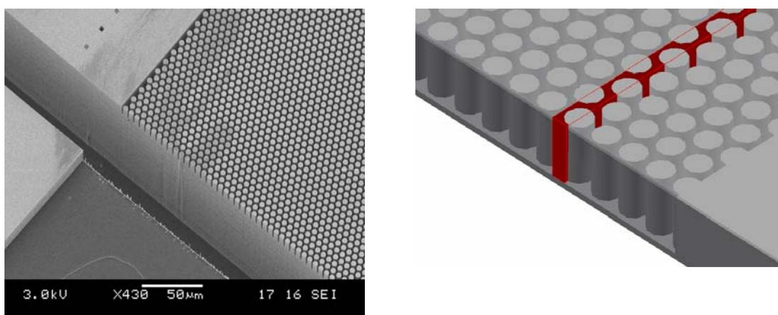
**Figure:** Overview of channel with etched pillars for HPLC separations and a computer-generated representation.
